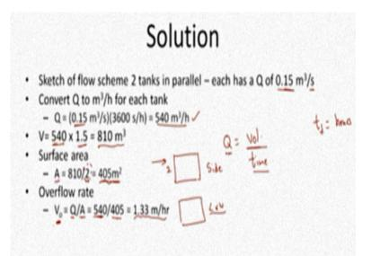
Well pretty simple calculations. Two tanks in parallel, so flow rate is half of the total Q from meter cube what we say convert Q to meter cube per hour for each tank. Looks like it was given in seconds but our time for detention was given in hours. If there are errors in the calculation that is fine you can just correct that yourself and volume is what is Q is equal to volume per time.
