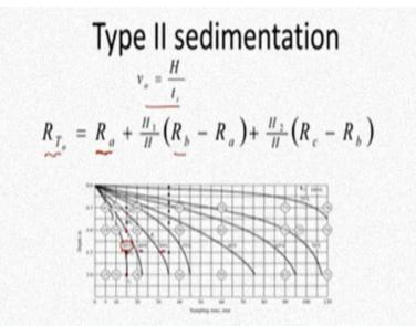
Overflow rate is given and how do I get that so that is going to be  $R_a$ ,  $R_a$  is already 30% for this particular case, total removal at that particular  $t_a$ , what is that equal to  $R_a$ ? 30% plus what is this H<sub>1</sub>, H<sub>1</sub> by H is nothing but the midpoint between these two particular points of intersection, H<sub>2</sub> is nothing but the midpoint between this point and this point.
