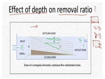
What is the effect of depth on the removal ratio is it? We have this basal and this is the relevant  $V_0$  and if  $V_s$  is equal to  $V_0$ , it will just be removed. If it is coming at the topmost location but, if it is coming at the bottom location not bottom less than the top when V s equal to  $V_0$  that particle will be removed.
