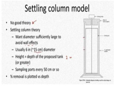
There is no good theory that is one aspect to keep in mind why is that if I am trying to design a segmentation tank, a new segmentation tank and if I want to look at the relevant design and I just want to look at it or come up with the design by developing a model why is that difficult because unless you have the actual waste water it is difficult to mirror it.
