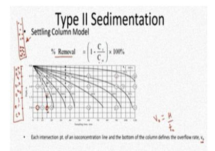
How am I going to plot it? Let me, let us just see here I have the different depths at which this is my vessel or my model and I have sampling ports at different depths and I am going to calculate the percentage removal in this manner  $C_t$  by  $C_0$  concentration; time t, remaining at time t and initial concentration let us see percentage removal will be  $1 - C_t$  by  $C_0$  into 100.
