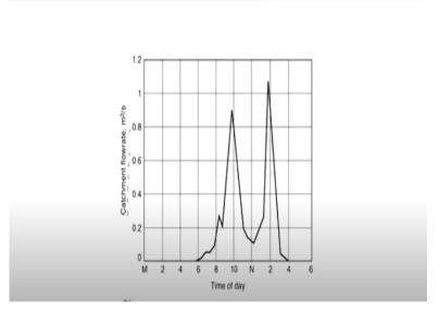
If you look at the hydrograph where we have the catchment flow rate, we see almost a similar profile being captured. You can see the relevant profile. The time scale is the same please note that. More or less similar profile means that the time for flow is relatively less. That is one thing to keep in mind. In other cases, the time will be can typically higher.
