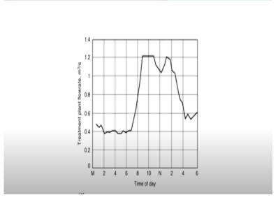
But for the same catchment area the wastewater treatment plant you see that the peaks are averaged outlets. That depends upon the flow coming in throughout the day and also the kind of sewerage network that you have and the kind of storm water control or diversion networks that you have. With that I will end today's session because I am almost out of time. But in the context of wastewater treatment, we understand two aspects or need to understand two aspects.
