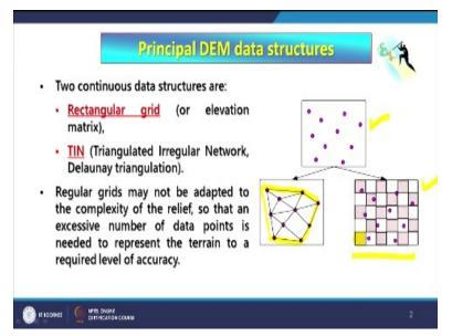
So, let us first try to understand what basically TIN is? As mentioned that both raster and TIN, are the continuous data structures. Raster; we have discussed sufficiently that is a 2 dimensional matrix of course, it is continuous. TIN instead of having unit in case of raster- a square, here we use unit as a triangle but the shape and sizes of these triangle are adaptable to relief changes and that is why the word irregular network of triangles is used here.
