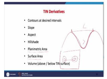
Now, what are the TIN derivatives? What are the things which we can derive from TIN? Of course contours; you can always drive because after all TIN is also formed using point data. The slope and aspect; these 2 parameters or 2 derivatives of a surface are simultaneously generated and then Hillshade can also be generated using your TIN model. And Planimetric area; this is very-2 important.
