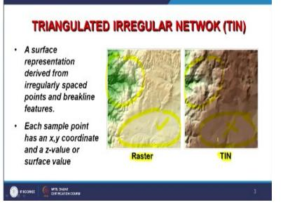
And it is derived from irregularly spaced points and break lines. Point is always input here if somebody is having poly-line data, no problem. Poly-line can be converted to point because after all poly-lines are also having series of X and Y's. So, we can convert or some smart software is capable now. If you provide input in poly-line, they will convert first into the points or use these nodes and internodes and create it in. So, that is not a big issue.
