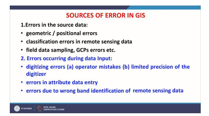
So, first one is Errors in source data. These we will put in under this category of inherent errors because we take lot of data from outside. And nowadays, lot of organizations are preparing data and providing which are completely compatible with GIS platforms or GIS software. If they do not declare that what kind of inherent errors are there then definitely, they are keeping users in dark and we may not be able to tell that how accurate our analysis is?
