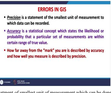
So precision is a treatment of smallest unit of measurement which can be done or recorded by an instrument. And another term which is accuracy. People many times take it synonymously which is completely wrong because these two terms are completely different. As you can see that accuracy is a statistical concept. Basically, it states the likelihood or the probability that a particular set of measurements are within certain range of true value.
