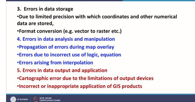
I was supposed to typed say 100.58 and I just left 100.5 so with wrong precision if I am not providing, it will carry the error. So, due to limited precision with which coordinates and other numerical data are stored especially this precision procedure will come with the co-ordinate. So, precision means here that to how many places after decimal, we will keep the data. Format conversion because any conversion from one format to another.
