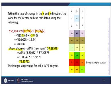
So, for taking all this together; X and Y direction, the slope of the centre cell is calculated using following formula, that now I am bringing X direction, I bring you by direction. Same concept; rise\_run. dz/dx, we have calculated 0.05 and where dz/dy in the earlier slide, we have seen is -
