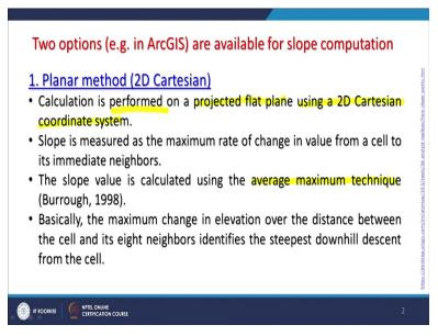
Basically, which calculates or perform on a project flat plain and using a 2D Cartesian coordinate system and that way, it calculates basically. So, slope is you know that it's a maximum rate of change in the terms of value. And slope value will be calculated for the average maximum technique. And this is what is there that average maximum technique which is calculated and basically the maximum change in elevation over the distance between the cell and its 8 neighbours.
