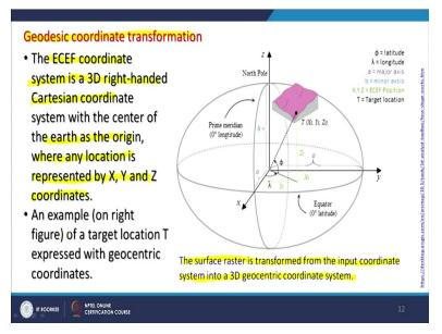
Now very briefly, I will touch about this geodesic co-ordinate transformation that is earth centre earth fixed one. Here because Earth is not perfectly spread so here it is little exaggerated thing for the Polar Regions. Just to explain that the surface is transform from input co-ordinate system into a 3D geocentric co-ordinate system, that is ECEF; earth centre earth fix co-ordinate system. So, whatever the input which is coming through the 2D, will go in the 3D.
