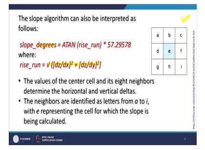
Now slope algorithm can also be interpreted as in this form like slope in degrees and where you know that rise/run will be decided based on this expression. And the value of the centre cell and its 8 neighbours like here in this example for each cell, the values are calculated and it will be in both directions. And neighbourhood are identified, here in this particular example between a to i which you are seeing; a to i and where e representing the cell for which the slope is being calculated.
