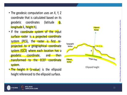
Now in this geodesic computation for x, y, z coordinates are calculated based on this geodesic coordinate that is latitude which is represented by  $\Phi$ , longitude  $\lambda$  and height h. So, all three are there. Now as I mentioned that more complications will come once you go for more accurate and accurate estimation of slope. Still, I am using word estimation because after all digital elevation model is a model. It is not a completely true one to one scale thing.
