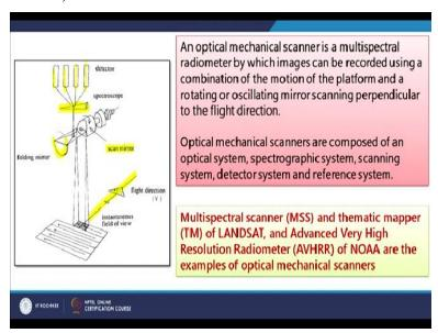
And similarly, a in optical mechanical scanners, so within these cross track scanners, there are little different options are also there. So, up to mechanical scanners, again these are multispectral radiometers and which can record the image or data or part of the earth using a combination of a platform motion and a rotating or oscillating radar scanning again perpendicular to the flight direction.
