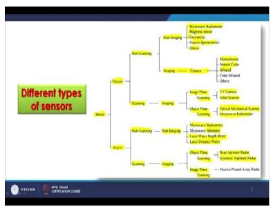
Now, it is specific to this particular discussion and different types of sensors are there have been there in on different kinds of satellites. So, we start with this kind of general logic that the sensor is there and there are 2 basic categories which we can divide these sensors, one is passive which is very common and other one is active which is microwave sensors. Now, in passive the we can divided in other 2 main categories.
