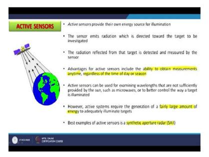
Now about active sensors, active sensors as you know, they are having their own energy source for illumination. And these active sensors emits send pulse or signals towards the earth target which they are focusing. And one important thing about active sensors and passive sensors, I should not miss here is generally passive sensors are neither local sensors or vertically downward. So, these satellites are generally looking vertically downward which we call is another viewing.
