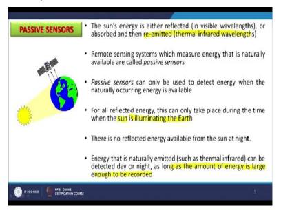
And these systems that passive remote sensing systems measures energy that is naturally available, that is why they are called passive sensors. And these sensors can only use to detect energy when naturally occurring energy is available and for reflected energy they need to have
