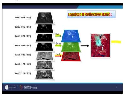
These are different bands on the latest example from Landsat and reflective bands are here only reflective band is there and not thermal infrared and thermal infrared channels are there. And, of course, we can assign different colors red colors for different bands as per our requirements and can create a false color composite like this or color combination like this as shown here.
