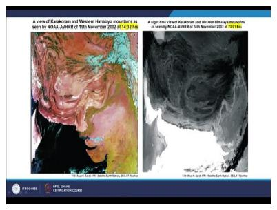
One example here is from NOAA AVHRR in previous lectures also with different reference we seen these 2 images, I am showing again this is color composite. And this is thermal infrared image of the same part, but it has been taken in the nighttime, but you can see here it is in the daytime. Of course, for the same day it also acquired daytime thermal infrared images also. So, they would that will look quite similar to what we are seeing is a 23 hours local time image of the same area.
