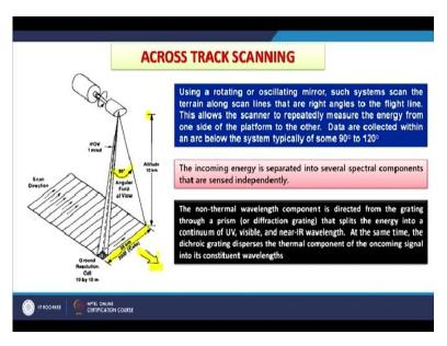
As you can see in the figure, that this is the path of orbit direction of orbit from where the satellite is coming and going in this direction and these scanners, they scan line by line which is across that track, there is the height which is given here and instantaneous field of view also is there, which we will be discussing in literal detail or later on and that also decides the spatial resolution.
