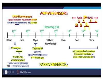
Now, where these sensors are located. This is very, very important and whether it is active sensors or passive sensors So these 2 extreme ends on the top we are having active sensors which are shown in red color. There is a in the bottom it is written is passive sensors which are shown in blue color and the EM spectrum here the part of EM spectrum is shown in the black and green color. So, we go one by one again, starting with the active sensors that we are having laser fluorescent sensors.
