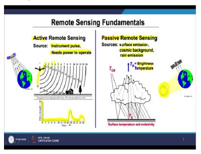
As you know that remote sensing we have just discussed that can be divided in 2 broad categories, one is a active remote sensing and another one is the passive remote sensing, what exactly is an active remote sensing means here that is the instrument itself since the pulse or the signals towards the earth and whatever the backscattering, which reaches after the interacting the energy which came through from the satellite towards the earth.
