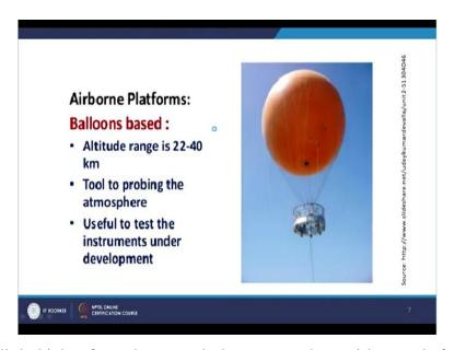
When we go a little higher from the ground, then we can have airborne platforms and starting with the balloons. So, balloons based very common, very old thing and it still it is being used that you can have a balloon, which can go up to 20 to 40 kilometer in height. And it can be used to probe the atmosphere different layers of atmosphere with different constitutes of the atmosphere depending on the what kind of sensors or payloads you are having.
