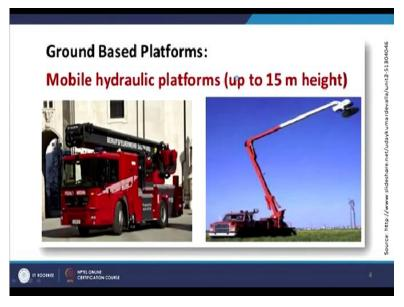
There are possibilities of using some cranes or some special platforms for collecting ground data like here one example shown is mobile hydraulic platform, which can go up to 15 meter height and you can have a payload on the top of this platform and then remote sensing can happen it is sometimes very useful in agricultural investigations or maybe investigation related with civil constructions also.
