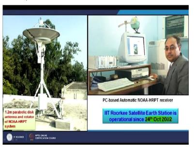
And this is the simple setup which we are having running and still data is being acquired this is external part which is a rotating or tracking here is a PC based system. And as mentioned it is working since October 2002.
