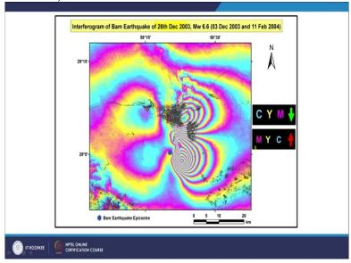
So, when we take this back again this interferogram of this now, we can interpret that in which part of a this interferogram the subsidence has occurred, in which part the upliftment has occurred between these 2 dates. And we know between these 2 dates, one big earthquake has also occurred. So, we can attribute very confidently that these ground deformations are because of that particular earthquake.
