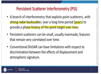
So, basically this is a branch of interferometry and that exploits the point is scatters instead of looking for you know and the fringes is here inducible points are used. So, point scatters are exploited with stronger radar backscatter which may be giving better or a strong backscattering over a long time period, that line time period might be years; because a lot of data is available successive data is available.
