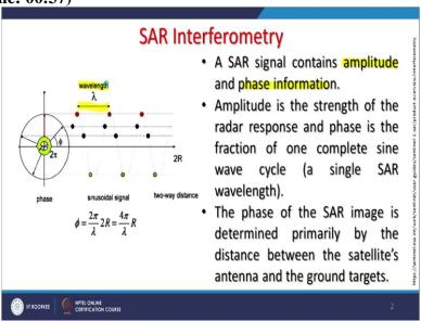
As earlier also while discussing microwave remote sensing active microwave remote sensing we discuss this figure, but very briefly I will bring that in SAR interferometry these SAR signals basically, as also discussed that they contain basically the amplitude and phase information and this amplitude and basically shows the strength of the radar response. And phase is the fraction of one complete sine wave which we are seeing here one complete sine wave cycle as a single SAR wavelength.
