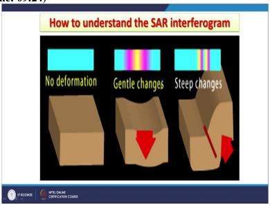
So, that way for example, this example we have seen little differently that when no deformation is there, like in this one on the left image, then and no fringes will be observed in interferogram, but it has some gentle deformation has occurred in this case is subsident, this is the pattern which will you will see and if steep changes have occurred, we might see even 2 fringes like here, the example here.
