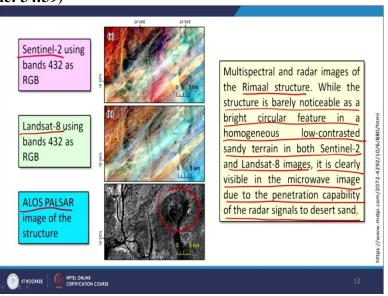
And the first 1 for the same area having different see here, the first 1 is from Sentinel 2 and this is of course not radar image. This is a band combination 432. These are multispectral images. The next one is also multispectral image, but the bottom 1 is the ALOS PALSAR image, which is a radar image and as you can see that these 2 top 2 examples from Sentinel 2 and landsat are giving though colors.
