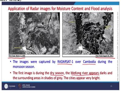
One more example and that radar applications of radar images for moisture content in flood analysis, as I have said that in case of flood the water is calm and therefore, there can be a specular reflection and then therefore the area may appear completely dark the flooded area
