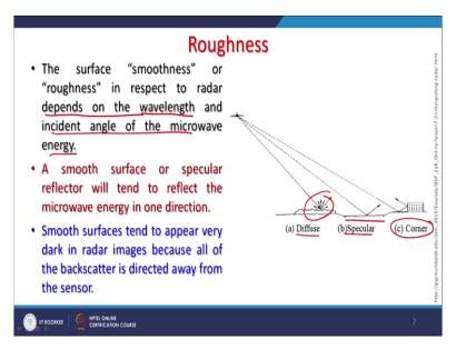
But also the incident angle of the microwave energy. As soon here that we may have a reflection like a diffuse reflection, specular reflection or a corner reflection and corner reflection that means, the maximum energy is going back to the radar. So, these corner reflectors the metal corner reflectors are used that is why they are designed in a manner that the maximum microwave energy is reflected back immediately to the antenna or receiver.
