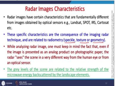
Now, these are a radar images have certain characteristics that are fundamentally different from images obtained by optical sensors. This I have been telling the radar images, interpretations and analysis of radar images is completely different than images which are coming from optical sensors, for example Landsat, SPOT, IRS, Cartosat etc. These characteristics or special characteristics are consequence of imaging radar technology.
