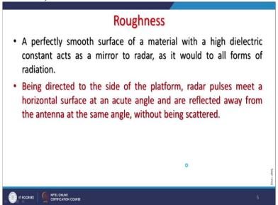
Roughness the surface roughness in a perfectly smooth surface of a material with high dielectric constant act as a mirror to the radar and it would be to all forms of radiation. So, they behave water body may behave as a complete mirror, because water is having dielectric constant, a smooth surface a calm water may behave like a mirror so, being directed to side of the platform.
