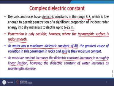
And dielectric constant in the range of 2 to 8, which is enough to permit penetration of a significant portion of incident radar into dry materials to depth of even up to 25 meter. In desert conditions, you do not have moisture in the sand. And therefore, because of a very little dielectric constant ranging from 3 to 8, which will allow the penetration and therefore, as soon as it encounters the water body.
