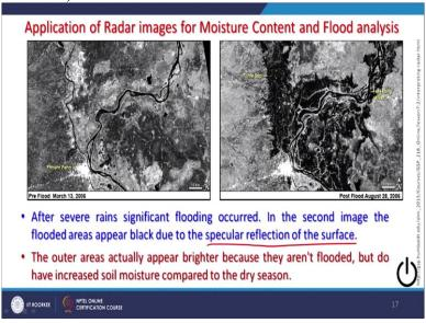
After a severe rains significant flooding occurred in this semi calm river and of course, the second image appears flooded and black due to a specular reflection of the surface. So, as we
