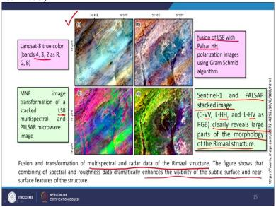
Now, as I was saying fusion of images, so, this is that example is here that that a is a true color image color composition band 4 3 2 have been arranged in RGB that is a part again of a desert area. And b is the fused image of landsat 8 that shown at 8 and has 8 PALSAR horizontal polarization. So, when you merged these 2 this kind of product can be generated,
