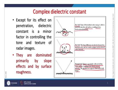
For example, in the soil, some of the incident radar energy is able to penetrate into soil surface resulting in less backscattered intensity. So, absorption is there, as you can see that some part is penetrating whereas, wet soil that means high moisture content and that means, large reflection because water content is more. So, the large differences in electrical properties between water and air results in higher backscattered radar intensity.
