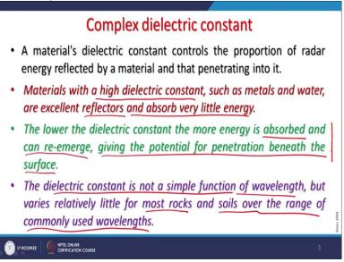
So, materials will the high dielectric constant, such as metals and waters and water are excellent reflectors and absorb very little energy and therefore, that is why I said that surface roughness of water also plays very important. So, they are also it will play a very important role. So, the energy which is not absorbed gets reflected. So, lower the dielectric constant more energy is absorbed.
