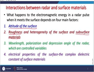
And basically depend on 4 major factors. So, when the satellite or sensors sense the energy or a pulse, radar pulse to the towards the ground and then the surface are the features which are present on the ground and will behave differently based on these 4 main factors. First of all the attitude of the surface how the surface is and how it is oriented, we have seen in case of a hilly terrain.
