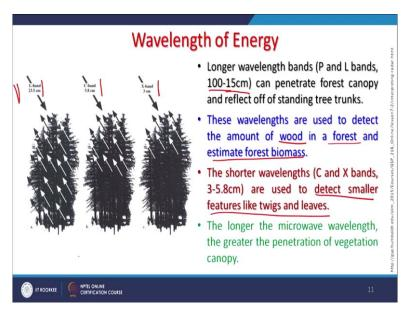
So, this is L band whereas, wavelength is 23.5 centimeter C band the second one middle example is C band 5.8 most common used in radar remote sensing maybe X band that is 3 centimeter. So, here in the L is having maximum wavelength X is having minimum wavelength in this example. So, what we see here that the white arrows are swing the back backscattering.
