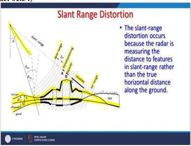
If we see here that this is the sensor and when the pulse is sent there are terrain is also shown here. This is the terrain and if there is a hill then first of all there will be a problem about the shadow. Because one side of the hill is illuminated, whereas other side is not illuminated and that will go in the shadow. And when we see these datasets or images, microwave power images, we will not see this part of the hill.
