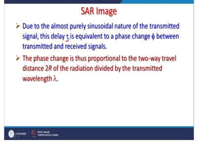
So due to almost purely sinusoidal nature of transmitted signal and this delay now is equivalent to phase change that is phi between transmitted and receive signals and the phase change is thus proportional to 2 way travel distance that is 2R. That is why in previous equation we have used 2R. So, the 2R of radiation basically divided by transmitted wavelength. Because the range has to travel twice, that is why 2R is taken.
