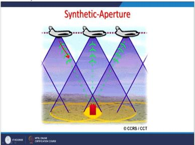
This is what happens exactly in the synthetic aperture radar that once the data is transmitted by a sensor towards the earth and then, as soon as the spacecraft aircraft moves whatever the backscattering is coming, it collects. And therefore, it simulates a large antenna in a space basically and that is why it is called synthetic aperture radar. So large antenna using the side looking airborne system, it is possible to create a large antenna.
