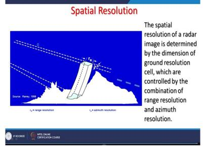
Now, how is spatial resolution is decided and spatial resolution in radar images is determined by that dimension of ground resolution or ground area which is covered by which is controlled by the combination of range resolution and azimuth resolution. So here and what we are seeing that in this case, this is the range resolution and here we are having azimuth resolution also.
