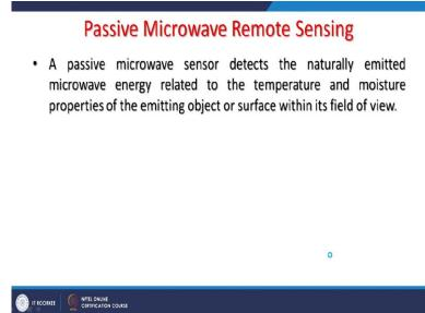
And basically detects that naturally emitted microwave energy and though this energy is very tiny, very small, and which is related to temperature and moisture properties of the emitting object. Soil or rocks are surface within his field of view. So, because the energy is tiny, then you require a large area to cover to register it is you know effects in the sensors those are which are very far or maybe 850 kilometre away from earth.
