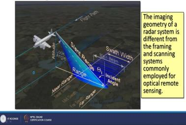
While seeing or analyzing active microwave data, here is the geometry and the spatial resolution and this is the slant range which I was mentioning, this is the flight path here and of course, the ground track is this one which is just vertically downward, this is the height altitude of the aircraft or spacecraft. Then the look angle that is there and this is what is the slant range if we go slant range is oblique obviously.
