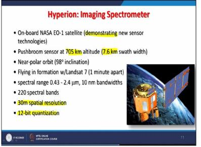
Earth Observing satellite one, which is demonstrating new sensor technology. The purpose of this mission was and the sensor is pushbroom sensor, and little older technology in that sense. And the altitude wise is 7.5 705 kilometre and swath but it is of course, about 7.6 kilometers swath width and near polar orbit as normal remote sensing satellites flying information with the Landsat and one minute apart so that we get coverage in multispectral as well as in hyperspectral.
