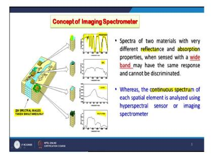
So, basically this imaging spectrometer and basically they started with the microscopic level, but now we have gone to an satellite base do like here this is the example of 224 spectral images taken simultaneously of different part of EM spectrum. And when these are you know different features are looked through like a first example is the water body, then this is how the spectral curve in different parts of EM spectrum one is going to have.
