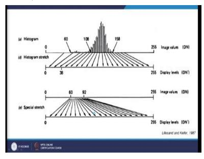
This is histogram equalization that we will be also seeing. So in histogram equalization, wherever the more frequency of pixels are there, they are more spread is there likewise.
