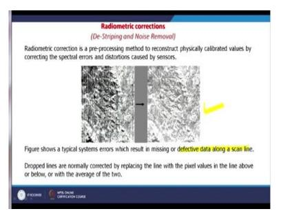
Like here the line which we saw was horizontal in the software here. The stripes are in the vertical direction but the technique would be same that adjacent pixels average value is taken and given to that drop line and you get a corrected image. Though, if we would not have the striping effect then the image would be different completely then what we are seeing here. But since we do not have any choice.
