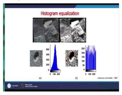
Histogram equalization can create a large contrast in your image compared to simple linear contrast. But which one would be best for your image for of that particular location of that particular day nobody can tell. So this is really one has to judiciously choose a right contrast stretch routine or you know tool. And then do it and try and see and assess how best the results are there.
