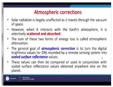
So that we are not here discussing when we will come on the radar data micro data then we would be discussing. Atmospheric corrections, we have already discuss and have done a separate treatment mean 2 problems in atmosphere scattering and absorptions and these can be a sometimes can be, you know can change the quality of an image very badly because of these phenomena.
