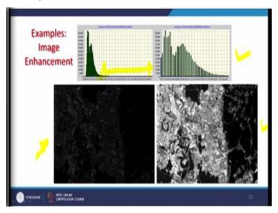
Now, one more example of real satellite images, when we see the raw images generally we see like this which we are seeing here completely almost blank. You are unable to see anything here, why because when we see the corresponding histogram of this image, the raw image most of the pixel values are very close to 0 or between up to 100 maximum. And this is an example of 8 bit image and we expected that the distribution of pixel values should be with 0 to 255.
