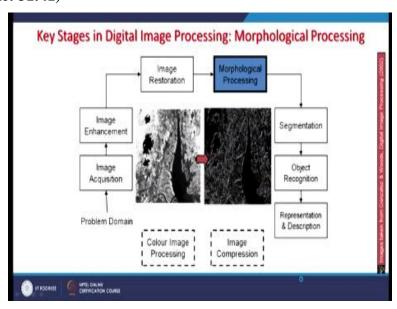
The next is the morphological processing like here I want morphological processing means spatial filtering which is done to enhance certain features or reduce the frequency of certain features. So for which morphological processing can be done, so this is on the left side is the input image and on the right side after morphological edge enhancement. So, edges of all objects which are present on the left side of image have been enhanced and it becomes almost a binary image.
