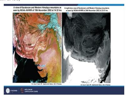
Now, since NOAA AVHRR sensors are having 2 thermal channels and therefore, it is possible to acquire data even in nighttime. This is not common with many satellites, because if they do not have the thermal channel, then the data cannot be acquired in nighttime. But NOAA is having thermal channels and this near infrared and 2 thermal channels 3 channels data can also be acquired in nighttime.
