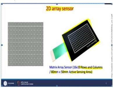
The real example is shown here, that matrix area sensors 16 by 10 rows in columns which is 80 millimeter and 50 millimeter and multiply by 50 millimeter which is the that active sensing area which is this much. Now, in compared to the linear area which we saw there will be heard and continue 2048 CCDs but here we are having just a few CCDs arranged and you say to them as and this is just an example of that.
