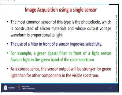
So most of the common one which we are having is linear sensors. Using single sensors and the image acquisition, the most common sensor of this type is the photodiode, which is constructed of silicon materials and whose output voltage waveform is proportional to light. So, they are
