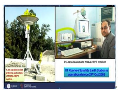
And this is one example of satellite earth station of NOAA series of satellites which at IIT Roorkee we are having and running since October 2002. It is having 2 major components, one is the external component as you are seeing antenna here and another one is internal component and which is inside the lab and which is just PC based system and the main here is the receiver.
