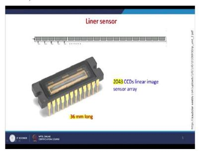
Whereas in case of line sensor you are having array of single sensors or CCD charge coupled devices arranged in a line and like here, this is the real photograph which is does just 36 millimeter long, the total length here and it is having to 2048 CCDs arranged in a linear. So, if
