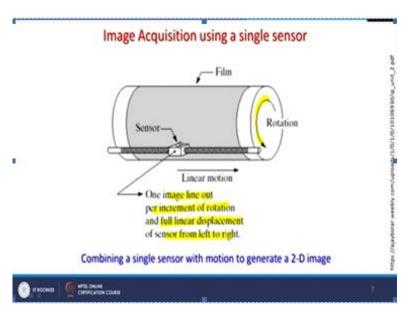
In case of single sensor when it is used and either only film sensitive or electronic sensitive devices when it is you are having a sensor it rotates, this rotation is there and it keeps recording the things. So, there may be a film or some other sensitive material. So, this is one image line out per increment rotation and full linear displacement of sensor from left to right. And such sensors are not there anymore now on satellites.
