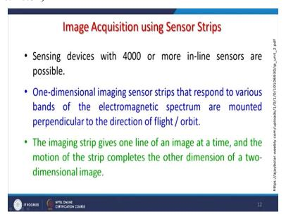
So, sensing devices with 4000 or more in line sensors are possible 2048 real example I also show to you. One dimensional imaging sensor strips and these you know areas and respond to various bands of electromagnetic spectrum are mounted perpendicular to the direction of flight. So, they are fixed devices, no mechanical things and their life is very good and very low and performance wise, they are also very good.
