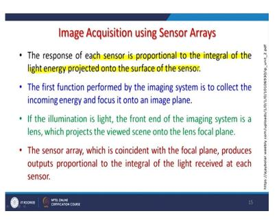
So, this is the response of each sensor is proportional to the integral of the light energy projected onto the surface of the sensor and the function of all these should be very much perfected. And there is the calibration part is most important in linear array or any such sensors or devices, sensing devices which are put on satellite images.
