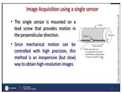
And the single sensor is mounted on a lead screw has shown here on the right side and provides motion in perpendicular direction and this mechanical thing is there and they are having their own difficulties. But trade office are inexpensive and one can acquire a high resolution images as well using even a single. So, low cost devices are possible.
