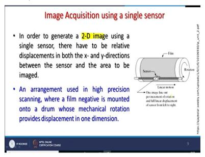
Whereas in case of this 2D linear sensor in case of linear sensors, a different scenario is there. So, even if one is having single sensor the 2D image can be generated by having this kind of arrangement of a rotating drum and line by line and that is the single sensor records the energy on the film or whatever material you are having.
