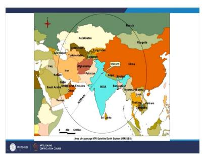
I will be showing an image also. But the purpose of showing this map is that it is showing the location this red dot is showing this IIT Roorkee satellite earth station and a circle is there of 3000 kilometer radius this is nothing but the footprint of a cone, base of a cone and whose apex is in the suppose 850 kilometers with the satellite. So, if anywhere if you project this 3000 kilometer radius circle in a space of 840 50 kilometer.
