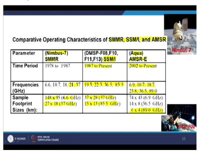
Now earlier there were many sensors where there are radio meters on various satellites. So, they were 1 satellite Nimbus-7, which had a sensor SMMR and that lasted between 1978 to 87. So, about 9 years it worked frequencies there between these ranges. And now the spatial resolution of footprint was of this size. So quite close resolution data. Then on this DMSP satellite again name you had this SSMI sensor or radio meter that.
