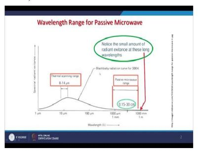
So, what we see here that this part of EM spectrum which is around 8 to 14 micrometer that can be used here. And as you can also see this is the spectral radiance existence and there we see that passive microwave. So, this part is for active microwave or sorry for thermal microwave and this part is for the passive microwave 0.15 to 30 centimeter and there the blackbody radiation curve for this one is also shown that is also shown here.
