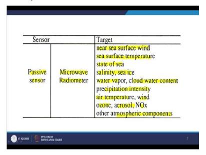
Like here this is passive microwave sensors. So, the main sensor here is the microwave radiometer and what are the targets or where it can be applied. So, near sea surface bands, there it is being used, sea surface temperature or SSD estimations it can be used it is being used and the condition of sea whether it is calm or very volatile that can be seen salinity also or sea ice, water vapour, cloud water contents precipitation intensity.
