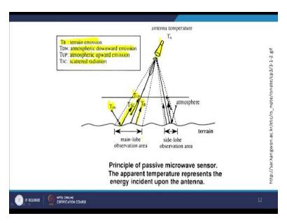
Like this is that horn is shown here. So, the main lobe of observation area and side lobe of the observation area. And so, this is the from the side the horn is detecting. This is from the directly is detecting and basically the TV, the TV component is the come in terrain emission a natural one and then there might be some reflected also and some other type of energy in microwave vision might be available like atmospheric downward emission.
