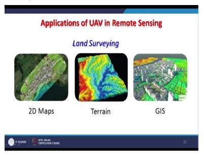
And these are becoming very, very popular and here few examples I can discuss which is directly related with how you UAVs are being used in remote sensing. So, first one is the land surveying of course, 2D maps can be created and the digital elevation models can also be created. These products are from there only. And the GIS or 3D mapping can also be done using UAVs.
