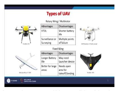
But the most modern one, the current one which are very light weight and very robust and it is very stable also. So, they are having either rotary wings or multi rotor are there are propeller. And of course, the advantages are that they are stable, disadvantage the battery life is a problem because all these motors have to run on batteries, sometimes, the loss of controls are also there. So, when you are having rotary wings these are the advantages and disadvantages.
