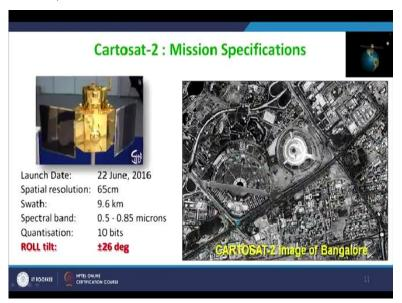
And in Cartosat, Cartosat became very popular because it has the capabilities this radiometric resolution was also very good and it has capabilities of acquiring data in a stereo pair and very much innovation was done and see the space of resolution. Now we are talking about 65 centimeter in Cartosat-2. So the best part here that for stereo images in a SPOT.
