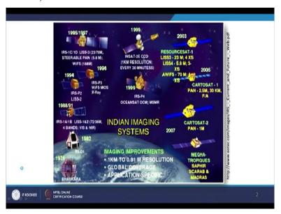
And that we are having a series of satellites as discuss also earlier but I would like to focus on this IRS-1A/1B and then IRS-1C/1D as you can see that and things have improved. They had 2 scanners LISS 1 and LISS 2 and a 72 meter and 36 meters space resolution in LISS three that things have improved 23 meter and 70 meter resolution and at the same time we also have a steerable pan at 5.8 meter resolution.
