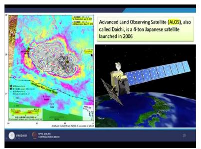
And similarly in the Sentinel SAR interferometry data has also been used. So, what here we are seeing on the left side is interferogram and interferogram which is showing of earthquakes, which has occurred in Nepal in 2015, which is on 25th April here on the left side and on the right side 12th May 7.3 magnitude. So, first one was 7.8 magnitude of 25th April and then 12 May it was 7.32.
