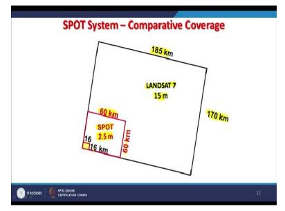
If we compare with the Landsat, the coverage, how much you know competitive coverage versus Landsat versus a SPOT, then this is what the scenario is that Landsat-7 is having 185 by 170 coverage or 1 scene will cover this much of area at 15 meters resolution, but when we go for 2.5
