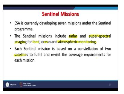
Now, we also cover one more very important mission which is Sentinel missions, there are now the Sentinel 1 and 2. So, these are very important data set and not only they provide the normal means these multispectral is cannot but they are also capable of providing interferometric radar data. So Sentinel missions include radar and super spectral imaging for land, ocean and atmospheric monitoring.
