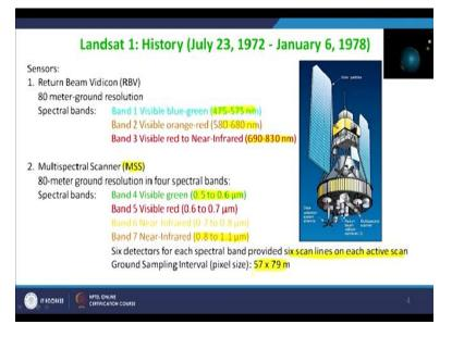
Instead, I would go on scanner systems on the Landsat-1. So, it has one scanner which is also used to call it Vidicon along with your MSS scanner. So MSS scanner was also there. So, in what we see that this RBV had 3 channels, visible, blue, green, and visible orange, red and visible red to near infrared and in different micrometer ranges are here they are mentioned in nanometre ranges where there and we used to call band 1, band 2, band 3.
