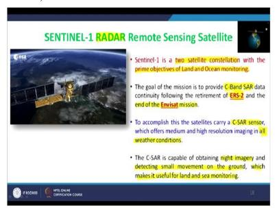
I will just focus more on the radar data because radar data used to be very expensive, but after the launch of Envisat and later on this radar sat or a Sentinel and this data has become free and very, very useful data for various kinds of studies. So, Sentinel-1 which is a 2 satellites constellation, Sentinel-1 A and 1 V with prime objective of land and ocean monitoring and the goal of the mission is to provide C band.
