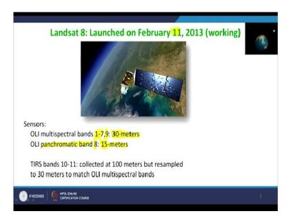
Now, the latest series which was Landsat-8 also call OLI series, which was launched in February 11 2013 still working giving good quality of data. So, there are more number of channels as compared to Landsat MSS. Of course, in between Landsat TM is okay. So, OLI is having channel number in the multispectral bands 1 to 7, then there is also 9 channel, channel 9 for band 9 and all are having 30 meter space resolution.
