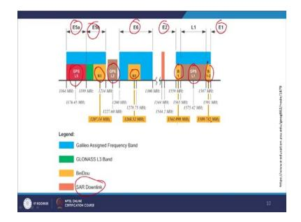
Now, for the comparisons that which navigation system or GNSS is fitting where which frequency they are using. So, say in that sense is a comprehensive picture is here. For as L1, you are seeing for the GPS as you can see here and for L2 also for the GPS and L5.
