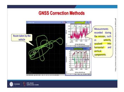
So, this is one of the examples that when survey was being done, this is how the track has been recorded and then the route taken by a vehicle or in air survey, a sortie have been recorded like this and later on through post-processing, one can make corrections and can make the data more accurate here.
