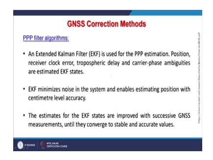
The filters are the Extended Kalman Filter which is used for PPP estimation and the position, receiver clock error, the tropospheric delay and carrier-phase ambiguities are estimated using this EKF states.
