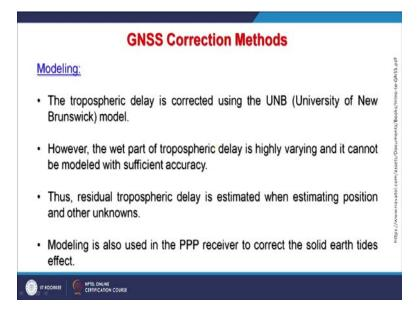
So, tropospheric delay is corrected using UNB; University of New Brunswick model. Generally this is the model people are using and however, the wet part where moisture is high of troposphere delays because of clouds and other. It is highly varying because you know the cloud keep changing and it cannot be modeled with sufficient accuracy.
