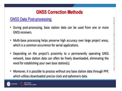
And during this post processing, the Base Station data can be used from one or more GNSS receivers. So, if there are more receivers which were involved in the surveying, all those receivers can use the Base Station data and corrections can be performed to achieve a better accuracy later on. Now multi based processing helps which preserves the high accuracy over a large project area which is a common occurrence for aerial applications.
