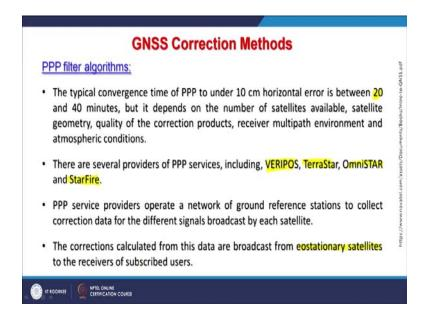
And the typical convergence time of PPP to under 10 centimetre horizontal error is between 20 to 40 minutes but it depends on the number of satellites available.
