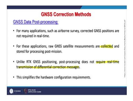
For many applications like for example, airborne survey corrected GNSS positions are not required in real-time. There can be many other services apart from this airborne service where real-time corrections are not required; means when the survey is being done either in the field or in the air then it is not necessary that at that moment I require the precise service.
