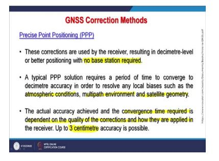
So, in this PPP these corrections are used by the receiver, resulting in decimetres level or better position with no Base Station required. This is the important point here that in this option that is PPP Precise Point Positioning System, the Base Station installed by the user is not required.
