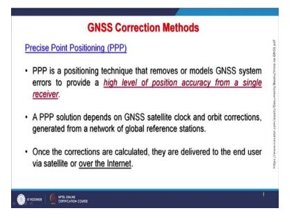
So, we can have a high level of accuracy from a single receiver. See maintaining 2 receivers; one stationary and one roving and then maintaining communication between them becomes very difficult and expensive option also.
