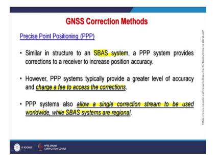
However in this PPP, which is quite similar to the structure or concept of SBAS systems which we have already discussed that the best part of PPP is that it provides corrections to a receiver to increase position accuracy. So, if I am getting signals from SBAS and using those corrections then I may not achieve that accuracy comparatively as provided through this Precise Point Positioning.
