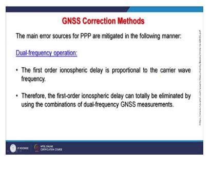
Now, the main error sources for PPP are mitigated by through these manners that the dual frequency operations because these receivers will receive signals in 2 frequencies. So, the first order ionospheric delay is basically proportional to the carrier wave frequency and those can be removed and therefore, the first order ionospheric delay can be totally eliminated by using combinations of the dual frequency GNSS measurements.
