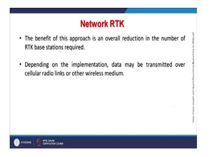
So, the network may be internet connections or through mobile network and the benefits of this approach is an overall reduction in the number of RTK base stations required. That is what people are targeting even a single Satellite Based Augmentation System can get better accuracy for you. So, depending on the implementation, how all this setup has been implemented, data may be transmitted over a cellular radio links or other wireless mediums.
