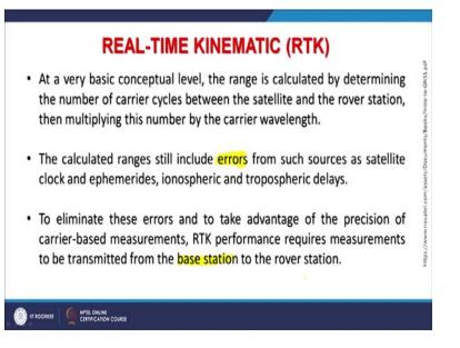
And the very basic conceptual level, the range is calculated by determining the number of career cycles between the satellite and the rover station and then using these carrier cycles to multiply this number by a carrier wavelength. And the calculated ranges still include errors which can be removed by using the base station data from such sources as satellite clock and ephemerides, ionospheric delays and tropospheric delays.
