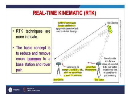
And these are the carrier phased measurements are being done by the base station which may be transmitted to the roving station in real time or a GNSS satellites can also transmit or a geostationary satellite can also transmit these errors signals to the rover receiver.
