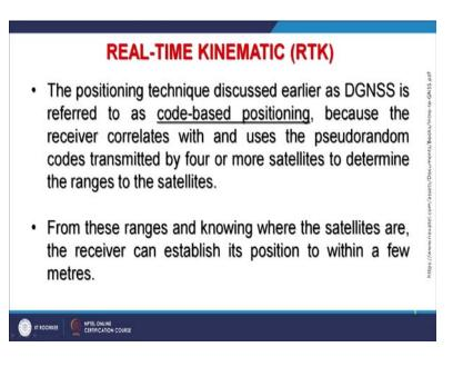
This RTK can become so useful and so easy that using a single handheld GPS receiver or GNSS receiver and even in your smart mobile can give you accuracy of few centimetres. So, that is the real future of this technique compared to DGNSS which is now it is already established that is there but you require different things setup for that.
