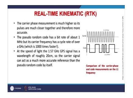
And carrier phase measurement is much higher. So, its pulses are much more closer as you can also see here and therefore more accurate it can give the position and the pseudo random code has a bit rate of about 1 mega Hertz but its carrier frequency has a cycle rate of over a Hertz which is about 1,000 times faster.
