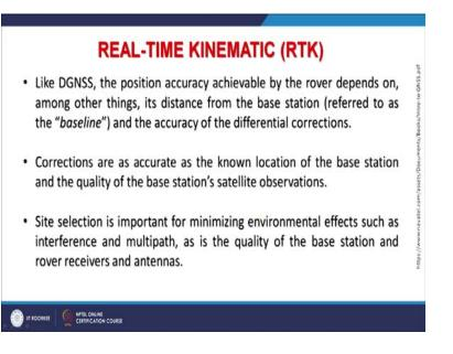
But if there is a SBAS signal which are transmitting errors then this problem can be solved. So, like DGNSS, the position accuracy achievable by rover depends on among other things, its distances from the base station that is a baseline and the accuracy of the differential corrections. Corrections are as accurate as known location of base station and the quality of base stations satellite observations and site selection is important for base station always.
