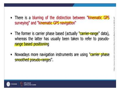
Now there is a blurring of distinction between kinematic GPS or GNSS surveying and kinematic GPS navigation. The former is the kinematic GPS navigation is a carrier phase based which is carrier ranged data which uses the carrier range data whereas the later the usually has taken the pseudo random based.
