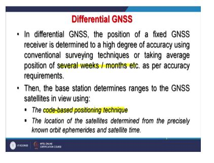
So, in differential GNSS; the position of a fix GNSS receiver is determined to a high degree of accuracy using conventional surveying techniques or taking average position of several weeks or months or it depending on how much accuracy do you want; in 24 hours sometimes it is also done. But more the data you are having, better the average would be and errors which you can use for the roving station would be much better and your accuracy requirements will also be fulfilled.
