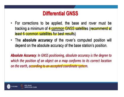
So, for corrections to be applied to roving stations data; the base and rover must be tracking a minimum of 4 common GNSS satellites. However, it is always expected that
