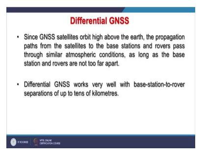
And GNSS satellites orbit high above the earth as we know the propagation path from the satellite to the base stations and rovers pass through similar atmospheric conditions as long as the base stations and rovers are not too far apart.
