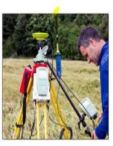
And once this information is there then it encodes this information into a standard format and transmits to the roving receiver in real time. And this is shown here complete setup of a differential GPS station and you can also see a transmitter is shown here, this is the receiver and these all controls are there.
