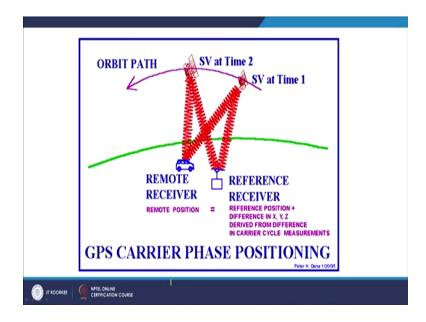
Now, because there are two ways of accessing signals or calculating the position; one is the code-based, another one is the career-based. So, we will be also looking in detail about the carrier-based system that is RTK; a Real Time Kinematics later in.
