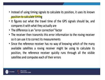
So, instead of using timing signals to calculate this position, it uses its known position to calculate timing and that is why it is mentioned that is a reverse process. So, it calculates the position to calculate to timing and this way, we collect the error information; those errors being received by our rover receiver. And once these errors information is available, we can subtract these errors from rover's position and can get accurate position.
