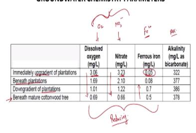
So let us move on so some of the groundwater chemistry parameters. So we are looking at upgradient beneath the plantation and downgradient of the plantation and also beneath the mature cottonwood trees now right. So here we have dissolved oxygen nitrate so o2, No3 and ferrous and (()) (33:12) let us say right. So again these aspects though if you look at it they will give an idea about let us say or the condition more oxidizing or reducing.
