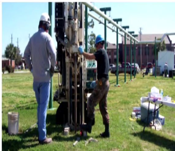
Retrieving soil cores using the GeoProbe equipment along transects extending across (perpendicular) the ground water plume
