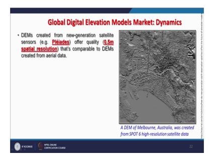
And this is the one example of that of Melbournes city of Australia which has been created this digital surface model here with this spot 6 and at 0.5 metre that is 50 centimetre spatial resolution. So, now, we are going some metre spatial resolution.
