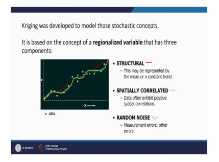
So, here now kriging was developed to model those stochastic concept, and which is based on the concept of regionalized variable that has three components all three together are here, but we can see one by one, that one is the red one is the structural component this may be represented the mean of a constant trend, or a spatially correlated component that is the data often exhibits possible positive or a spatially correlations, or random noise which is also soon is through a zig zag file.
