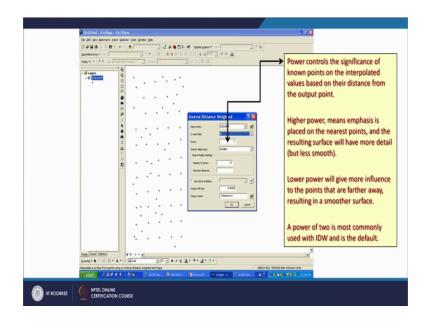
And for example here this is the example from a very popular gis software, which is arc gis arc map, and here the some soil sample data is being displayed which is randomly distributed, and a the method of interpolation has been choosing is IDW, and here what we are seeing that the pH value for we are considering as a z value for creating a surface, and a the number of points which will be searched around a unknown point are a in this particular example are 12.
