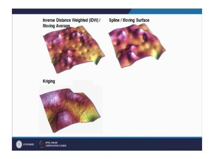
So, here using different techniques an example is shown, that using the same data point data sets same data point data has been used, while creating a surface using IDW method, then here sp line method and the kriging method, you can see that how completely different surfaces have been created using three different completely different interpolation techniques, though IDW and sp line are producing a little closer surfaces, but krig kriging surface is altogether different.
