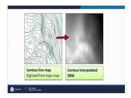
represented and the same contours can be used to create a surface that is nothing, but a digital elevation model, and this is how it will look.
