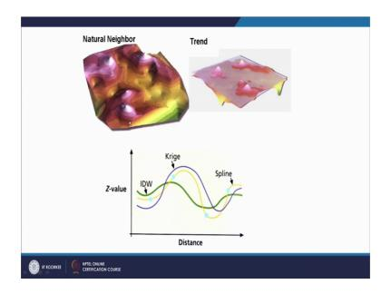
Instead of seeing surfaces like here if we see a profile of all these threes surfaces, and also locations of observation points point data is also shown, what do we find here? That IDW is the surface is going like this in this schematic and whereas, your a this sp line surface that is in yellow color is a absolutely fitting with all data points, and where is your krig surface is going above and lower of these.
