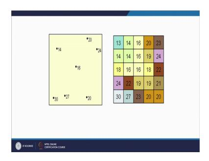
This is the example here that randomly distributed some elevation points are here, using these points a regular grid or a digital elevation model can be created, these lines say or this grid of lines and rows and columns are just shown for our understanding, but in a real digital elevation model boundary of each cell or boundary of entire dm, is not a really there except just for our understanding this grid of or biomass has been used here for our end.
