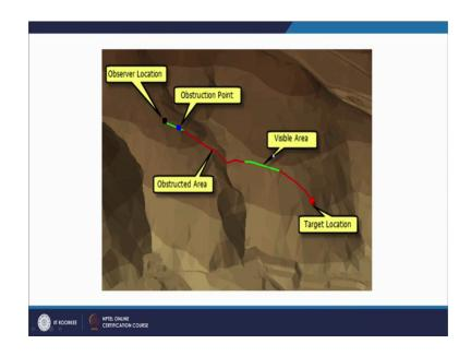
Again along in line this is example from digital elevation or tin triangulated irregular non-network on which also we can perform the same view shed analysis. This is the example here that this is the observer location this is the target location which part would be visible. And which are given in green colour which part will not be visible are given in the red colour. So, the input can be either your digital elevation model that is raster or can tin also
