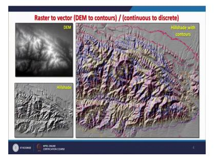
So, here also and this is the hill shade; one of the derivatives we have already discussed how these are derived, and the top of this hill shade on the right side what you are seeing the contours. And I will just show you that how contours can be derive using a continuous, its a reverse process.
