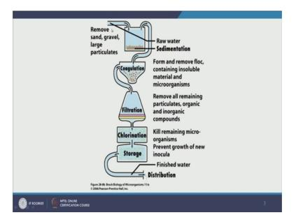
So, here first step is removing sand gravel and other large particulates. And once that has been done by sedimentation so, we allow these heavy particles to sediment, because they are heavy they sedimentary easily.
