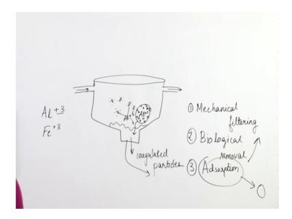
So, a typical coagulant is a salt of aluminum with triple electrons that it has given away and ferric, which is called alum this is a typical coagulant that has that is used in most laboratory and many drinking water and water treatment systems, where we use the coagulation process to get rid of smaller particles.
