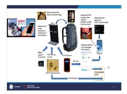
Now these sensors sends different kinds of contaminants this sends what were they there was battery for supporting the sensor there was a pump, but PM 2.5 pump based on cyclone movement what it would do it was collecting here and measuring real time amount of PM 2.5, there was a UFP DISCmini which measured other kinds of contaminants kept the information stored it into sd card.
