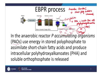
Now, this is what your typical EBPR process would blow you have first passing it through an aerobic chamber and then through an aerobic or anoxic chamber. And then you have a clarifier which is secondary settlement tank and then a part of it is returned activated sludge and a part of the it is wasted and then there is affluent that you send for disinfection. So, there is a disinfection step here and then you dispose it in the environment.
