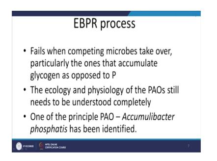
There is a major limitation with EBPR process which is that it fails when the competing microbes take over. So, in this case when the PHAs are degrading lot of energies being produced out of carbon is being released. So, biomass is increasing and if instead of our poly PAOs which are phosphate accumulating organisms.
