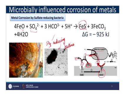
So, here you have a heavily corroded pipe and this is a sulphate reducing bacteria.
