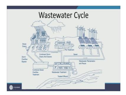
So, this is a typical wastewater cycle. Here, we have establishments. So, we have houses and industries or shops commercial areas and then each house each commercial area is producing wastewater. At times we also collect the sewage, not only sewage but also kitchen waste and also the storm water. So, storm water is the water that falls from the precipitation rain and it is a runoff; surface runoff.
