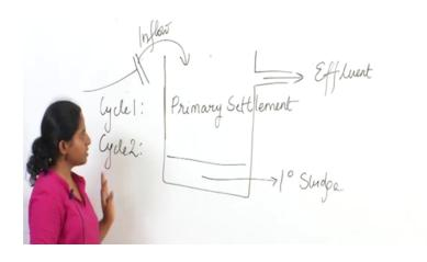
So, your SBR, our sequencing batch reactor will look like this. It is a singular tank. So, unlike PFR, when you have multiple tanks for different steps and the entire batch moves from one time to another, much like a train the compartments of a train. In a sequencing batch reactor, everything happens in a single tank.
