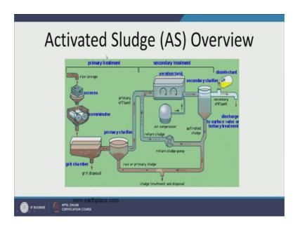
This is a PFR based process and we will quickly go through this. The primary treatment would include receiving the Rossi ways and then screening it to get rid of the big particles and particles that can destroy your wastewater treatment plants such as, aluminium forus and you have a communater, which breaks them into small pieces and then you have a grit chamber, this is where the grit is allowed to remove.
