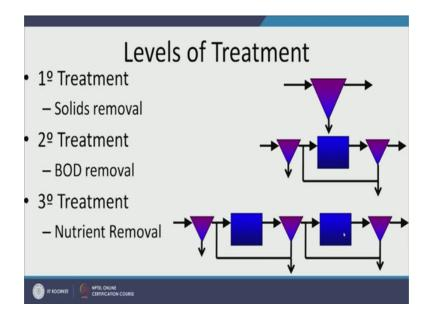
Now, let us look at the levels of treatment. Primary treatment, physical process we remove solid, then we can add to primary treatment, we can add secondary treatment, where we are trying to remove biodegradable organics or BOD and then you can add third degree treatment. So, this is primary, this is secondary. BY third degree, we are trying to remove nutrients from the wastewater already.
