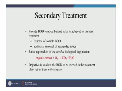
So in secondary treatment, we are trying to remove BOD, beyond what be removed in the primary treatment. So, in primary treatment, whatever could settle, the habit particulate matter - BOD has been removed, but the soluble BOD remains. So, this needs to be removed and then it also removes the suspended solids in the water. The basic approach in secondary treatment, that I have mentioned before is, aerobic oxidation of biological aerobic oxidation.
