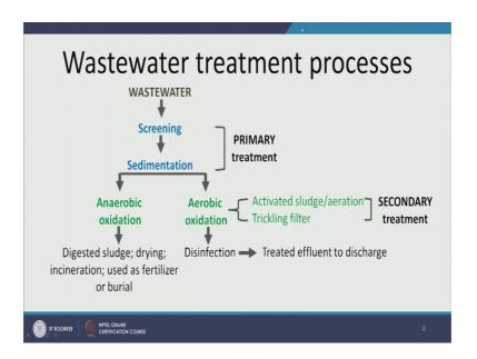
So, the wastewater is collected from different parts of the city or the area or the region that comes under the waste purview of the wastewater treatment plant and then it is taken to the wastewater treatment plant. Now one thing I wanna mention in most developed countries that I am familiar with usually there is a pipe system like how we had drinking water distribution system there is a wastewater collection system, that that is also laid at the time of constructing a city planning a city.
