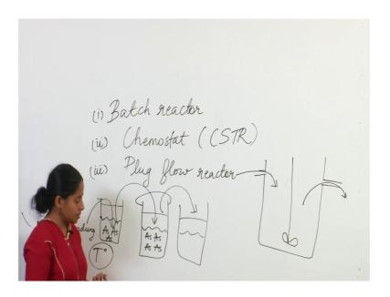
In continuously stirred tank reactor our reactor looks very different; it will typically have a port for entry of reactants continuous entry of reactants and another port for continuous exit of products. So, we have a infield and then usually if it is chemostat or continuously stirred tank reactor, it will go continuously, it will undergo continuous mixing.
