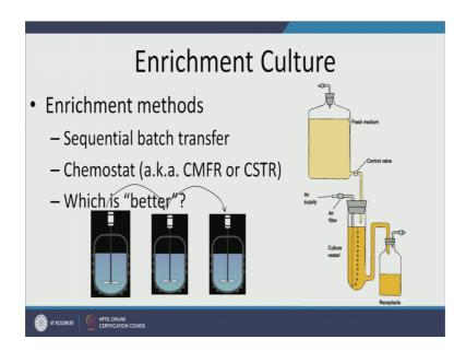
So, in chemostat this is your reactor, this special tube it has a continuous air supply, you can oxygenate it if you want to enrich aerobic microbes, or you can make it anaerobic by purging it with nitrogen.
