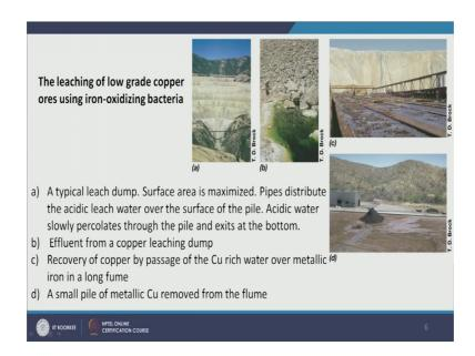
So, these are other pictures from USA and they are from the origin look there by the original Doctor Brock researcher. So, here you have low grade copper ore that is being leached out using iron oxidizing bacteria. So, in many a times copper and iron many copper and iron ores actually co exist. So, this is one of those mines and this is your typical leach dump and here we try to maximize the surface area and thus we have different steps as you see here.
