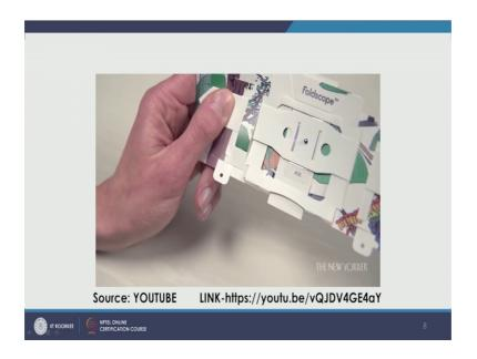
So, it is a flat sheet of paper you fold together and you have a fully functional microscope in a couple of minutes. It weighs less than ten grams and in the end you get an instrument that can give you 700 nanometer resolution imaging at a price point of roughly a dollar. Eco systems are not just based on large species; so, when I walk in the forest I am not just looking at the big trees but I am also looking at the fungus and the insects crawling around.
