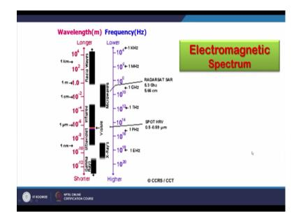
Now you will see in the tile different parts of the EM spectrum so let us start with here there are different sections are there and name of some satellites are also given for which the data we process like SPOT HRV is their dots red SR is there. So the radar sides occupy the part of the EM spectrum of that microwave section and were spot Millie focus is in this visible part.
