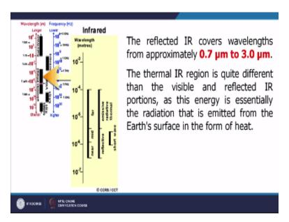
And the reflected infrared covers 0.7 to 3 micrometer and the thermal infrared region is quite different then of course the visible and reflected infrared portion as this energy is essentially the radiation that is emitted from the earth surface in the form of heat. And as mentioned earlier that any objects on the surface of the earth which is above epsilon 0 a natural condition will emit energy or heat and that can be detected by sensor which are having currently.
