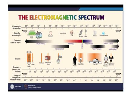
And how you know the different wave part which is section EM spectrum are shown, some example radio waves which are used for our radio transmission other purpose is announcements and other things microwaves is another one field which is very common then infrared this will part is occupy a very small portion of entire EM spectrum then you are having ultraviolet light and X – rays and other thing.
