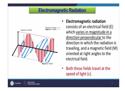
The magnetic field is shown here with the blue color electric field is shown and the red color in the simulation one can clearly understand that how both of these fields travel together but perpendicular to each other. So electromagnetic radiation of an electric field that is E which varies in magnitude in a direction perpendicular to the direction in which the radiation is travelling and a magnetic field oriented at the right angles to the electrical field.
