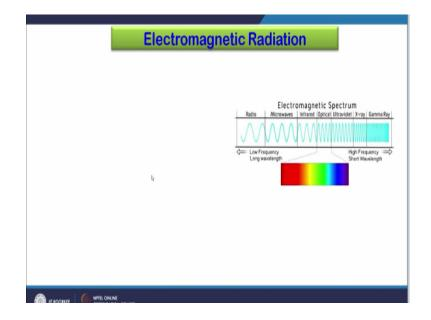
So the frequency is normally measured in hertz, equivalent to one cycle per second, and various of hertz. Wavelength and frequency are related by the following formula. And that is  $c = \lambda v$  and this  $\lambda$  is the wavelength v is the frequency cycles per seconds and the c is the speed of the light which is 3 x 10<sup>8</sup> and the shorter wavelength the higher the frequency the longer wavelength, the lower frequency.
