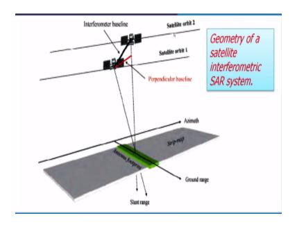
That this is the orbit one a1 after 35 days again the same area is covered by but by two different angels and this is the perpendicular based line, this is another very important factor that closer the orbits 1 and orbit 2 are, the smaller the perpendicular base line better the interferometry would been able to create because we could code and in these two images and likewise this is the data and is required.
