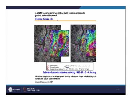
The subsistence is taking place that subsidence the example here the Kolkata city. And subsidence can also be measured. That how much subsidence is taken place. So if you are having a time difference of five year time difference satellite image is of microwave region. You can create an interfere program in see that what is happen in last five years for during the period. So in this one can estimate that how much ground deformations, Because of over withdrawal of ground water has taken place.
