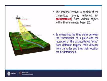
and the antennas receives a portion of a transmitting energy reflected or backscattered from various objects within the illuminated beam by measuring the time delay between the transmission of a pulse and the reception of the backscattered or echo from the different targets their distance from the radar and thus location can be determined.
