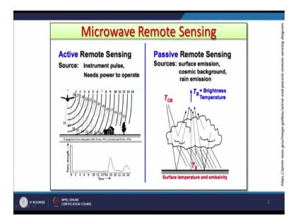
Where the signal is sent by the sensor itself and the back scattering comes it is collected by the receiver and then images are formed and where as we en can see also that the pulse is sent and then return whatever is the left or back scatter which is also received so likewise line by line pixel by pixel images formed but the image which we see in optical or near infrared thermal infrared the construction of those images is entirely different then in microwave.
