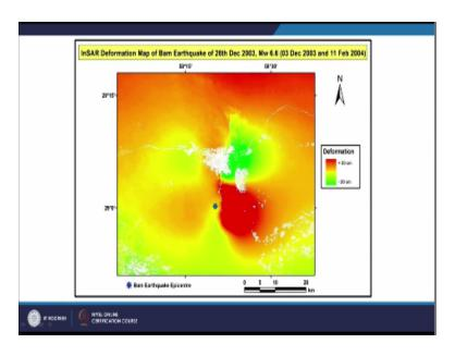
So this the deformation map and now it is the line of side, now this is in vertical component which we are talking. So there is up liftmen as I was mentioning here and this was the position of the epicenter so there is a up liftmen in this particular case was 30 cm in the – of the due to the earthquake and there where the subside in this part of 20 cm. so then you can say the half meter, the total half meter deformation on the area uptake place to that earthquake event.
