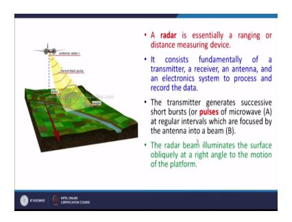
So this is how it creates the image here in this one we can see that the here though which is a hear bone sensor bud does not matter the same thing happens in case of satellite that they did and the signals are transmitted and then in the blue curves you have seeing the back is scattered which is going back and this is how different targets so different objects on surface of the behave differently in microwave region.
