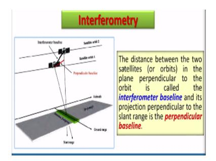
And the distance between the two satellite sheer or in plane perpendicular to the orbit is called interferometer baseline or and its projection perpendicular to this is the interference meter base line and this is the perpendicular and it is the perpendicular base line this is more important for interferometer now the asp programmed is generated by cross multiply.
