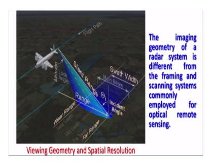
So this is the slant range, this is the range on the horizontal plane and this is the ultimatum, with this triangle this is the slant range and this is the incidental angel main been the coverage area, or swath width is that much, so we also say far range and near range, so the imaging geometry of a radar system is different from the framing and scanning systems commonly employed for optical remote sensing.
