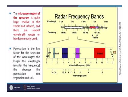
This is the different bends of frequency bends which are bold in microwave and as you can see that there is an X band there is a C band S band L band and some other bands are here so the most popular one are X band and C band which belongs to part of microwave region so microwave region of a spectrum is quite large not like visible in infrared there you are having the very small part of the spectrum level.
