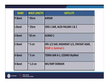
So like a the first microwave length is fully operation satellite by ERS one and later which is ERS 2 and that was in the C band RISAT in the Indian one is also a C band satellite and the C band is also on the sentinel which is European satellite and providing data free of cost to a users so thus the biggest advantage with sentinel and the data is available for the C band that X band is also in TERRA SAR a COSMO-skymed there are K band which are Military domain not in civilian domain.
