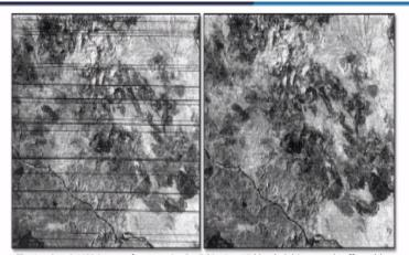
The Landsat-2 MSS image of an area in the Ethiopian Highlands (a) is severely affected by lines of spuriously low data. In image (b) the spurious lines have been replaced by, data derived from those in the adjacent lines. At the scale the defect is hardly noticeable.
