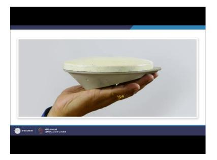
Let us say this is an example, this is an antenna where you can say the shape is dome shape and inside it is a circularly polarized which it is specification will tell, you will not be able to see from outside. Moreover for very precise GPS surveying actually you should go for still better type of antenna which is called known as geodetic geo free antenna.
