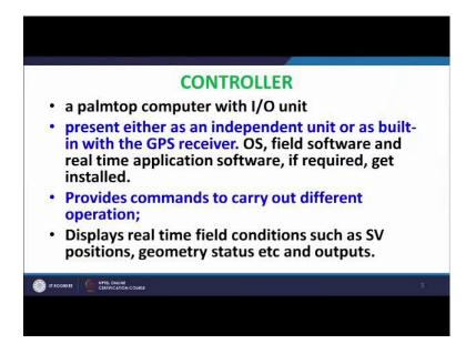
Let me now discuss on controller which is nothing but a palmtop computer having input output units. Now commercially the controller may available in different forms like it may available in an independent way. That means, it is independent of receiver as well as antenna or it may be associated with receiver or it may be integrated with receiver as well as antenna.
