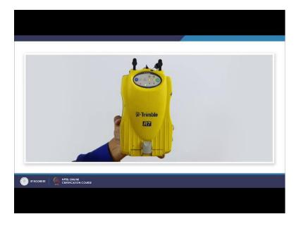
Now here is a GPS you see where which is being used as an independent unit for GPS survey. So, GPS receiver we may get either as an independent unit or it is associated with the other parts.
