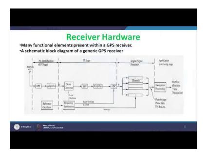
Next the GPS receiver hardware; actually as I told you GPS signals are very low in power as well as it get merged with interference from the higher powerful signals. So, we need to improve the power or in the signal as well as we need to filter the interference as well as we need to for the process the signal to get our desire parameters. In order to get those things the GPS receiver hardware contains filters, amplifiers, frequency unit, digital signal, processing unit.
