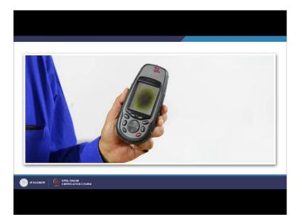
Now, let me show you one of the single code GPS receivers that would generally use for the recognizing survey is this one. However, there are hundreds of varieties of single code GPS receivers are available and most of the GPS enable mobile phones are also associated with C A code or single code GPS receiver.
