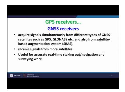
Now this type of receivers may receive signal from any combination like it may receive signals from GPS and GLONASS or it may from GPS and Bido or some other combinations. Now these types of receivers are most robust because they provide us information from different radio navigation system. So, there will be more much more useful for specifically for navigation purpose, air navigation purpose and real time staking out work, etcetera.
