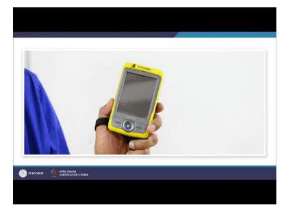
So, like these we may have now as I showed earlier this is a unit where antenna GPS receiver as well as controller having input unit, output unit is put together. It is an integrated GPS receiver. So, we get different types of controller were also available in the market.
