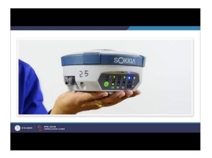
So, again this is antenna which is connected to GPS receiver, but controller is not associated with it. Now there are different antenna available in the market which is independently available which we can make use along with receivers and controller by using some connectors.
