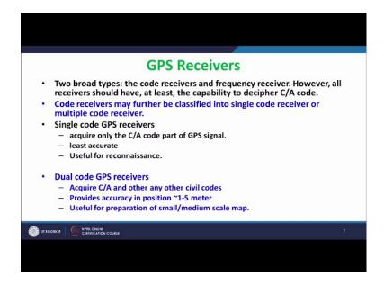
Now, let me discuss on GPS receiver as a whole. That means, I want to really take into antenna, controller, as well as receiver hardware together to work as GPS receiver. Now commercially there are different types of GPS receiver available and depending upon the accuracy how much it can achieve we classify the GPS receiver in the perspective of surveying into two types. One is that core type another is the carrier type.
