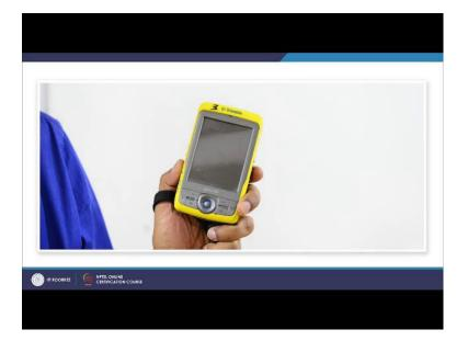
This is another GPS receiver where also antenna is embedded inside this case along with the controller as well as receiver.
