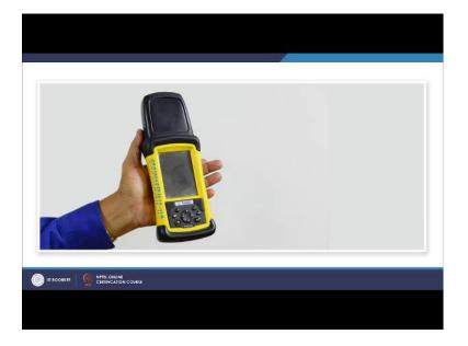
This is also a controller, where GPS receiver associated with it. So, it is an integrated unit of receiver as well as controller.
