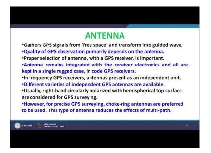
Now the antenna is used for gathering the GPS signal out of the lot of many electromagnetic signals that are available in the atmosphere. Once it gathers it transfers the signal to the GPS receiver hardware. Now the quality of the GPS signal that depends on the characteristics of the antenna which we will be using along with the GPS receiver. So, the antenna to be selected for use with along with GPS receiver is very important.
