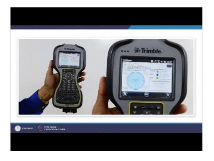
Let us show some example. Now this is a controller where the computer this is the input unit and this is the output display unit and this controller has to be connected to antenna as well as to receiver independently, though connector using this input output ports.
