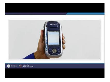
But, this is a controller also it is attached with receiver. Though it looks like same as before one, but it has GPS receiver associated with it. So, receiver as well as palmtop computer as well as the input device and output display unit.
