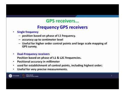
Now let me discuss on frequency GPS receivers. Now again frequency GPS receiver may be of different types depending upon how many frequency it can decipher. However, all frequency receivers in the beginning first it will decipher the C A code, from C A code only it will get the identification of the satellite from which the signals are coming and also it will get the time.
