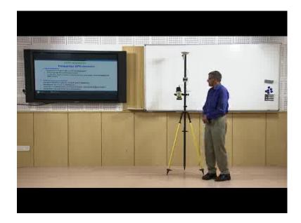
Let me now demonstrated you the single frequency GPS receiver. Now here you can see a receiver where this is the antenna and this is the receiver and this is the controller. Receiver and controller are together and they are connected to antenna using a connector and they are mounted on a tripod stand. If we take these arrangements outside this room in open sky then through this antenna we will be able to get the GPS signal and recorded through this GPS receiver.
