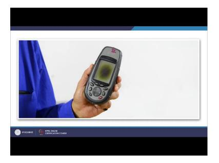
Now, let us take this case this is a GPS receiver where antenna is encased with in the same framework of the electronic hardware along with receiver and controller.
