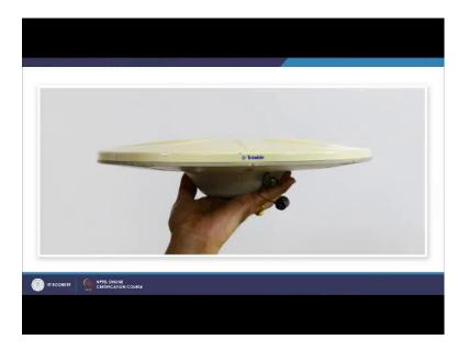
Like this one, where this is an antenna also again for GPS surveying and this is being used for very precise GPS surveying where the top of this is also a dome shaped and it is
