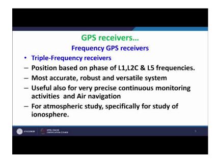
Next I will discuss on the triple frequency GPS receiver. This type of GPS receivers receives GPS signals and can decipher signals of L1 C A code, L2 C A, as well as L5 signal.
