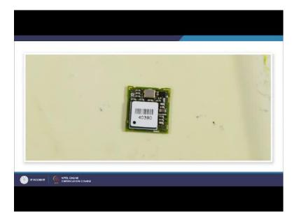
Now, I can show a small GPS chip. This is the GPS receiver chip which is used to make some instrument using GPS receiver.
