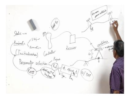
So, let us consider, suppose we want to set up our instrument somewhere here. So, we have to place the tripod stand of the antenna in such a way that it is centred then the antenna is to be placed over it so that antenna face centre is antenna face centre should be just above the station and we need to know the height of this antenna face centre above
