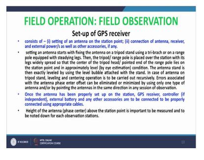
Now that is called setting up of the GPS receiver. In during our setting up of the instrument also we should note down the height of the antenna from the station point.
