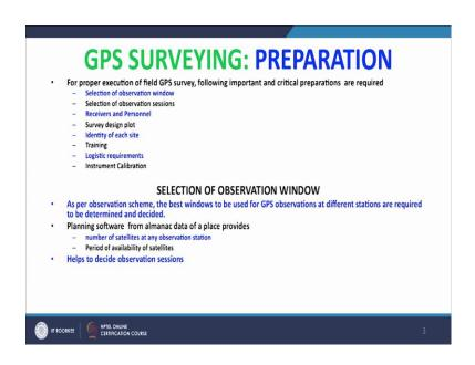
Now, the GPS satellites are revolving around the earth and the satellites are constantly changing the constellation of the satellites are constantly changing. So, we need to know at any instant of time during our observation how many satellites are available, which are those satellites, what those satellites are and how these signals will be coming all those
