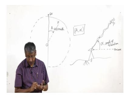
Now, what is that? Actually if we take a receiver like this, now this is the satellite from which signals are coming. Now if we say that this is the horizontal line then this is the line of site so this is called angle of elevation and if we see in a planimetric position and this is the position of our receiver O and this is the location of the satellite P.
