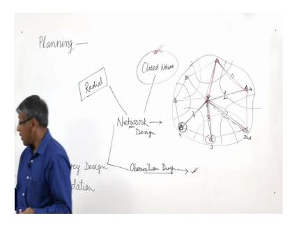
Now in case of GPS surveying the survey design consist of 2 parts; one is that to develop the network of the stations. How these networks are to evolve the stations has to be placed in the project area, and that is called network and the observation design. That means how the receiver has to be placed in different station points during observation. If
