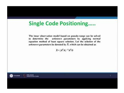
And this linear model has been used to find out the unknown parameter X, the position of the receiver by using least square analysis normally equation method and we have end up with this.
