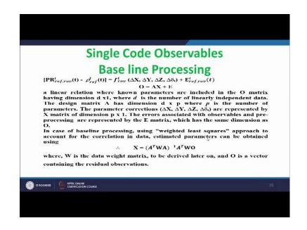
Similar to this, in case of baseline processing also we had ended up with this relation. So, this is the non-linear equation that is based on single code GPS observable for baseline processing. Now since this is a non-linear method. So, using the identical way what we did in the single code point positioning this non-linear model first has to be linearised
