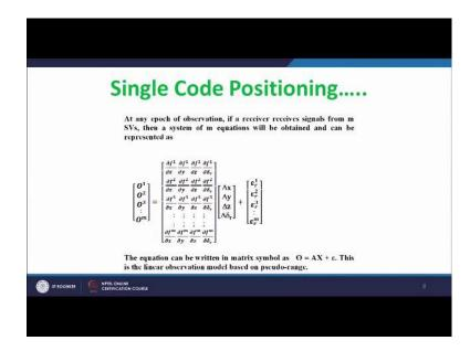
So, now you can see here that this is the observable equation that we get or the linear model we have developed out of the observation equation. So, here the observable equation for a single satellite, now the signal coming from a single satellite - this is the observable equation linear model and for m satellites this is the relations we have derived in the last class. So, which can be converted to this - this is the in matrix notation and this is the linear model.
