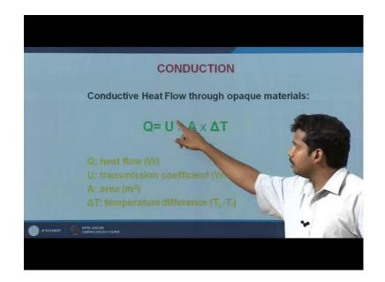
On one side you have Q which is the conductive heat flow through opaque materials which is equal to U, U is a transmission coefficient. We are going to look at this particular number more in detail U which is a heat transfer coefficient conductive heat transfer coefficient. Area of the surface that I was mentioning about how much area is involved in the heat transfer and the temperature difference delta T.
