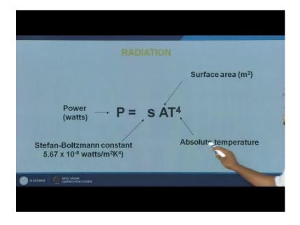
Radiate heat transfer can be calculated, you need a Stefan Boltzmann constant then the surface area and the absolute temperature of the emitting surface.
