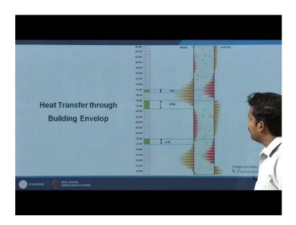
Let us take a look at this particular image. There is a cross section of a wall; it can be any material for now we are not getting into what are the thermal and physical properties of this wall. There is cross section imagine it is 200 mm thick wall and here what you see is the time line, its starts from 12 o clock on a particular this a night, then it goes on to the 1 day cyclic 24 hours and then this is a second day
