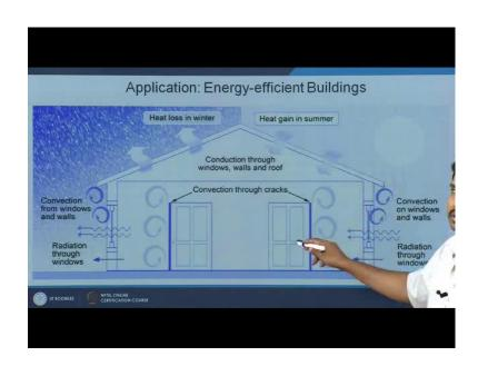
What happens through the wall simple conduction phenomena that will looked at first it can happened through wall, it can happen through window, it can happen through roof or through the ground there can be conduction. Then the next thing is convection, where it can happen through open window or it can happen through mechanical system or it can happen through cracks in the doors and windows.
