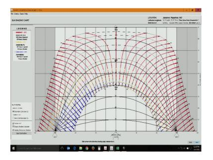
It can display a shading calculator you can actually you know adjust to what season you need shading. Specific shading design and calculation I will cover in another module, but this has a provision to adjust and you can actually move the shading mask. You can also specify obstructions whether the obstructions are there in which orientation and in what height we will look at the sometime later in the module.
