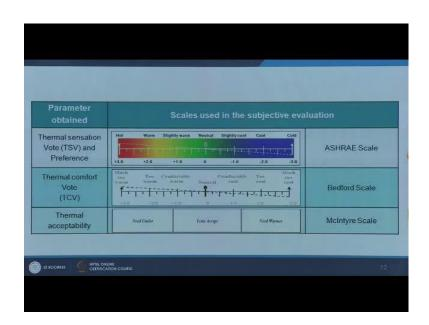
So, primarily these adaptive studies revolve around conducting field measurements of comfort it has two components, one is physical measurement accompanied by subjective assessment. It is like you have a set of sensors you go to the field you measure the condition parallel you also ask people, how do they feel? So, how do we ask how do they feel and what do you measure this is what you are going to look at this section.
