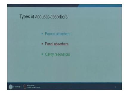
There are three types, primary types of acoustic absorbers; first is porous absorbing material, second is panel absorber, and the last is cavity resonators. Each one has a specific band width or frequencies spectrum, in which they have a very good performance. It can be stretched out to other frequencies, but their primary performance areas are different.
