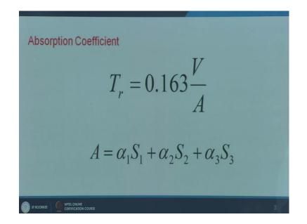
So, if you have n number of materials spread over specific surface areas, then you can have a sigma that is specific absorption coefficient, which into in the surface area. In this particular number a, is referred in terms of absorption, is referred in terms of Sabin; that is a unit for absorption. Now we will look at more closely about what this alpha actually means
