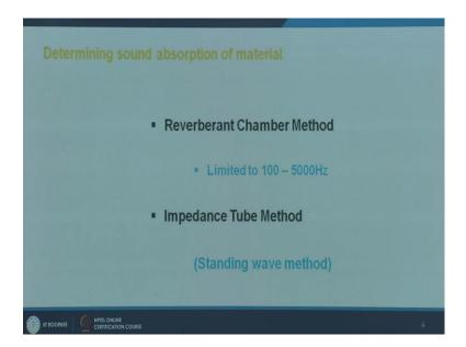
Alpha is the absorption coefficient of a particular material, it ranges from 0 to 1; 0 is 100 percent absorbing 0 is 100 percent reflecting; that is does not have any specific
