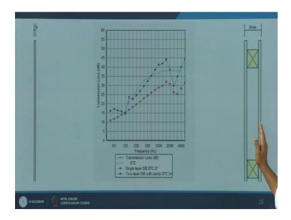
Getting certain specific examples, let us take a single layer of gypsum board, a thin gypsum panel; say around 30 in mm or 50 in mm gypsum panel, this is a absorption you know sound transmission class, or the sound insulation property at different frequency, the red one, this is what you are going to get. Now if you add a cavity at two specific gypsum boards, you are trying to increase this particular number; the STC value from 27 you are able to achieve 34.
