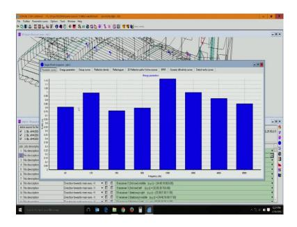
T 30 that is reverberation time 30 d b d k, these are specific frequency, you also get this for t 20 t 15 early decay time; t 30 looks like this. Then you also get different parameters like curvature, sound pressure level. This is definition d 50, this is clarity 7 c 7 c 50 c 80, we were discussing about c 50 and c 80.
