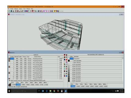
Next comes, the material specification. So, if you take a typical material. We are going to talk about absorbing materials later typical material, depending on frequency you see in this left hand corner, there is a material library from which we can choose, or we can add materials, depending on frequency the materials absorption considerably varies.
