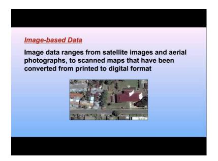
Whereas in case of image it might be having reflection value, or emitted value, or temperature value, or any other value is represented there, but in satellite images since this is coloured image; therefore, it is constructed using three primary colours, and therefore, you are seeing in colour, but still all are raster, and different type of raster which is a your image raster.
