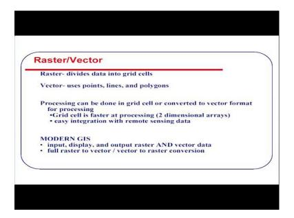
As we know that raster which we have already covered this part, the raster divides into grid cells vector uses point line polygon, units in case of vectors are point line polygons, in case of raster, either cell or pixel. And this processing can be done with grid and convert it from vector to raster, and all modern GIS software supports all three types of data handling.
